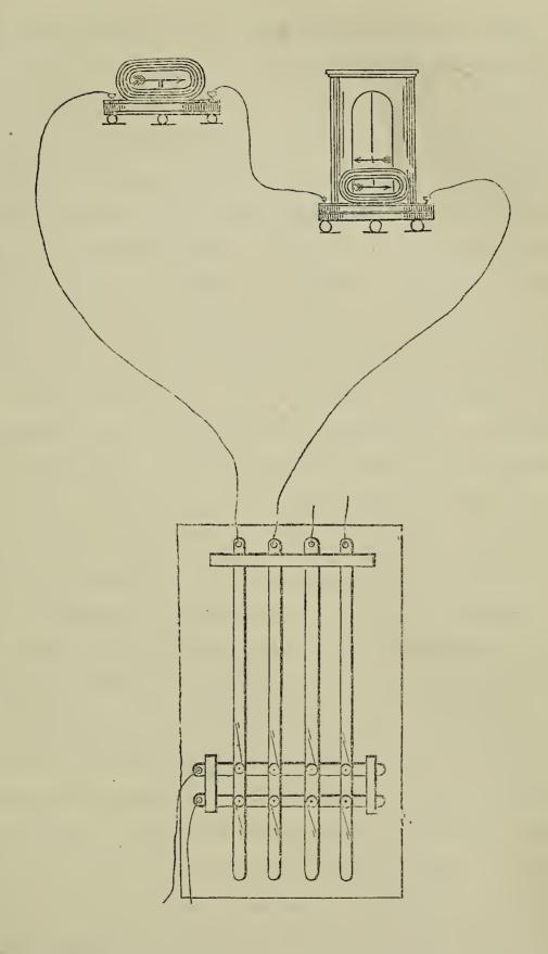
Plan of Professor Wheatstone's Permutating Key-board, being his only telegraphic instrument at the commencement of the partnership: shown in connexion with a Melloni's galvanometer, and a common coil, used in his experiments.
